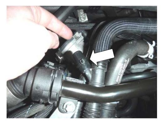
11. Using the short hose provided, connect the OEM breather hose to outlet port on the catch can.
