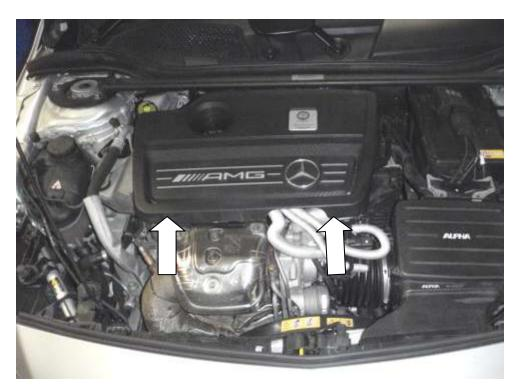
3. Using an E14 Torx socket and suitable ratchet loosen 1x bolt on the bracket at the rear of the engine. Do not fully remove the bolt only undo it enough to fit the 3mm bracket behind.
