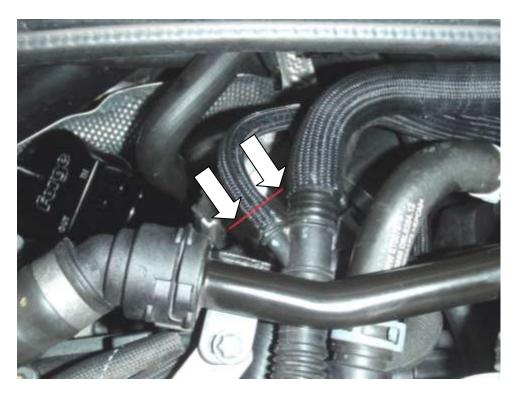
10. Using a sharp knife, cut the remaining piece of hose away from the plastic spout. Slide the silicone cap over the spout and secure in place with the cable tie provided.
