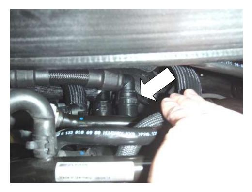
13. Push the crankcase breather hose onto the 8mm spout. Use a suitable lubricant if required and secure with the remaining cable tie.
