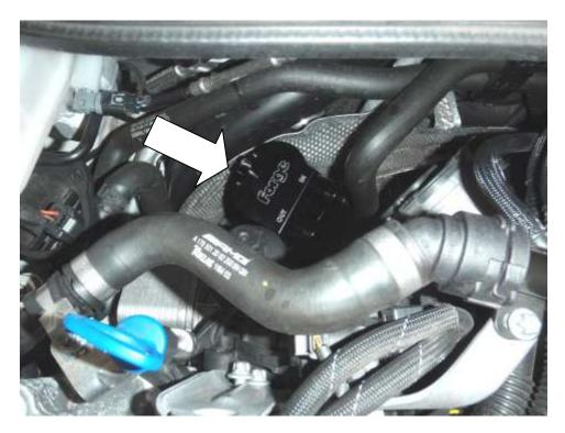
5. Secure the bracket provided with the M6 x 20mm Allen cap bolt, 6mm washer, bracket spacer, 6mm penny washer and M6 Nyloc nut.
