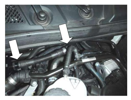
12. Connect the remaining hose to the cam cover outlet and the inlet port on the catch can.
